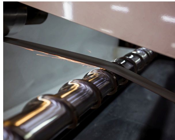
Pictured: grinding of feed screw
