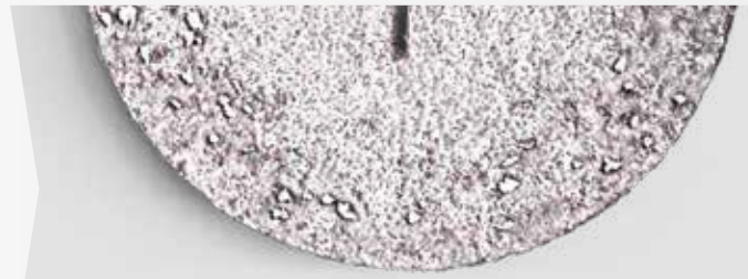
VSM ALU-X: It is clear to see that significantly fewer chips stick.
