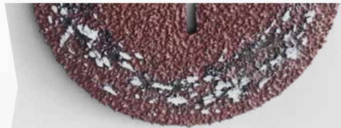
Fiber disc clogged with aluminum chips
