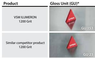
\*The **Gloss Unit (GU)** is the measuring unit of a gloss meter. A zero (0) value represents a perfect matte finish, while a value of 70 represents a typical high-gloss (high-shine) surface.
