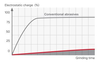
Significantly reduced static charging when processing non-conducting materials
